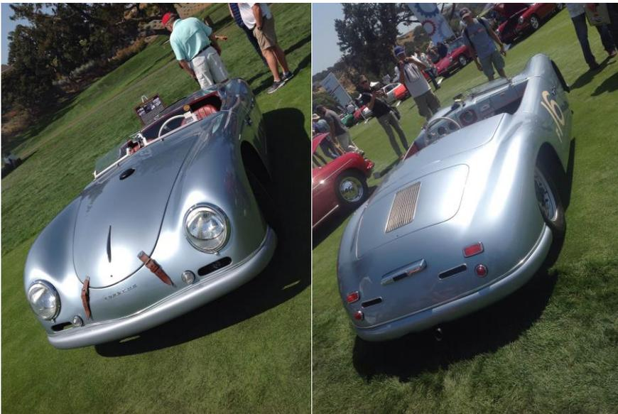
The Sauter Roadster with chassis #10359, weighing in at about 1350 pounds, went on to be the first 1500cc Porsche with Type 528 engine to race Nurburgring. Design wise, it inevitably influenced many factory production models continuing into the 1950s.
