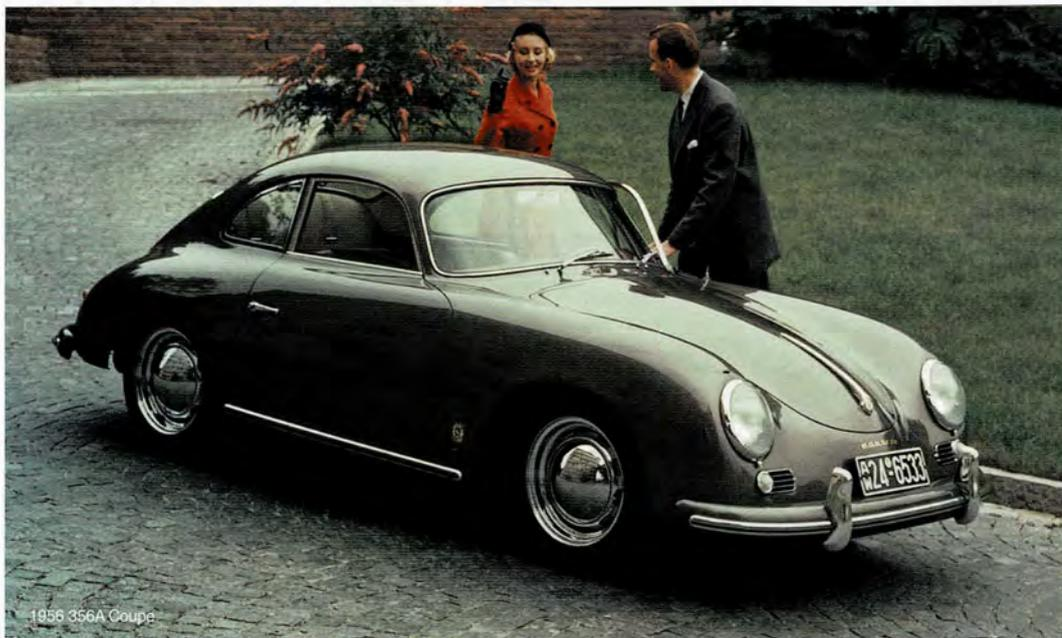
With Ferdinand Porsche's close connection to Volkswagen, and the difficulty of obtaining new automotive components in post-war Germany, it's little surprise Ferry looked to the Beetle when designing the 356. On paper, the list of similarities between the two models is striking: unibody construction, rear-engine/rear-drive layout (and a VW-derived engine), torsion-bar suspension, and so on. The reality was a bit different, however.
